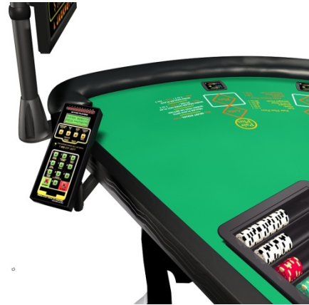
Figure 3: Installed Dealer Interface
