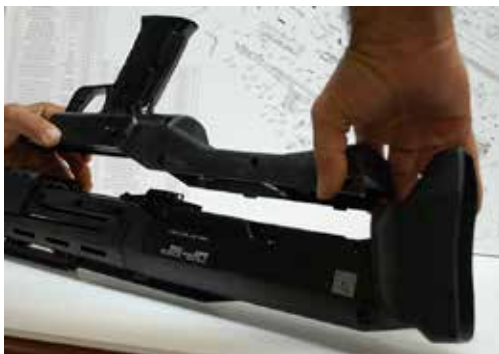
Figure D-8: Pull rear away from aluminum action.
