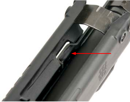
Figure E-1: Ensure Bolt Carrier is Locked into Forend
