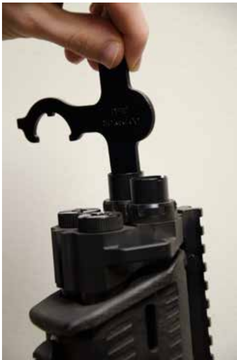
Figure F-1: Turn counter clockwise to remove choke tubes.
