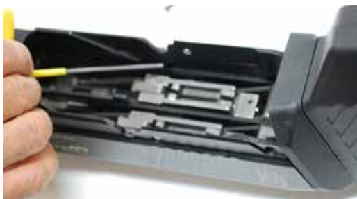
Figure D-13: Remove Exposed Bolt from Receiver
