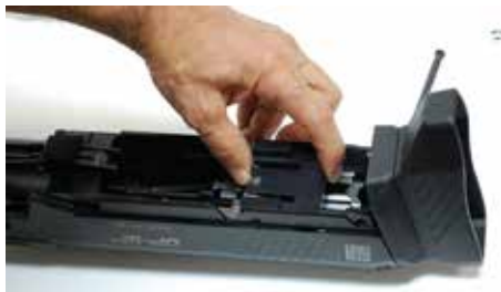
Figure E-4: Slide the bolt retainer plate down through the cutout
