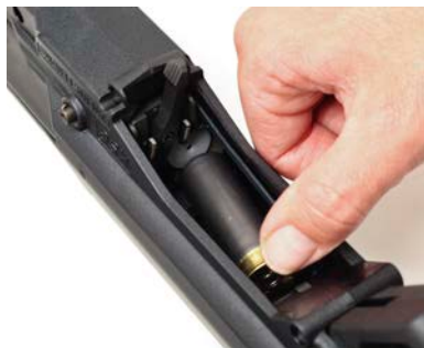
Figure C-2: Loading a Shell into the Magazine Tube
