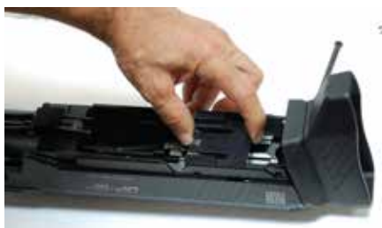
Figure D-10: Slide the retainer plate forward and lift up and out.
