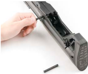
Figure D-2: Place Rear Assembly Pins in Retaining Holes
