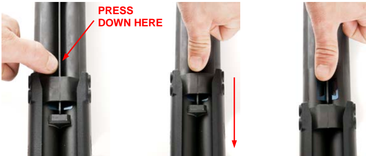
Figure D-7: Press down CTG Stop Actuator and Slide Forend Away
