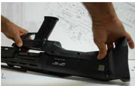
Figure D-7: Remove grip assembly
