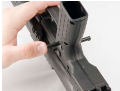
Figure D-2: Place Rear Assembly Pins in Retaining Holes
