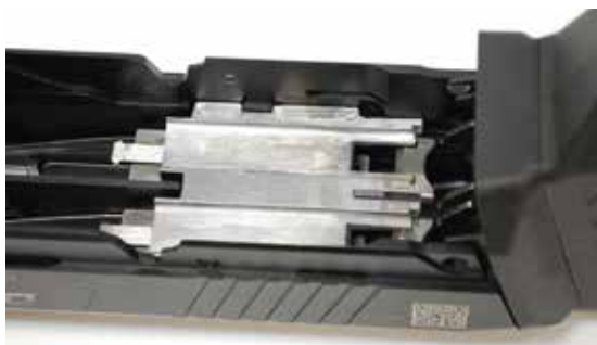
Figure D-11: The bolt and bolt sled resting in the receiver.
