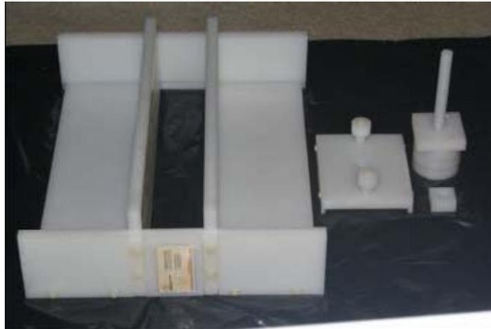
Figure 2: Sampling device frame, slide, weight and nut
