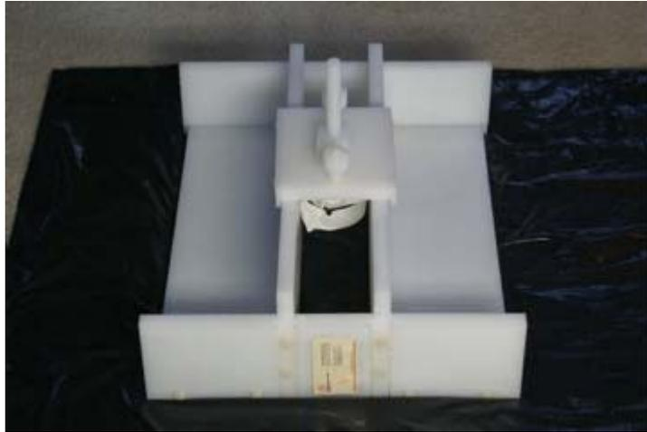
Figure 5: Slide placed on device frame rails.
