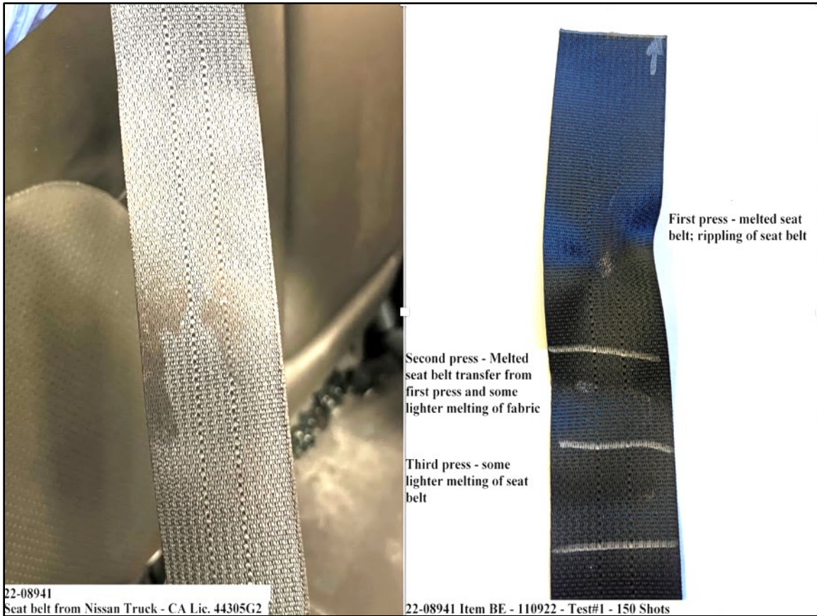
Photographs of the burn mark on the seatbelt of the Nissan (left) and test seatbelt (right). The image on the right shows three areas where the Daniels Defense rifle was test-fired; notes by the criminalist refer to each test-fire as a “press.”
